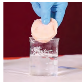
Green Rhino® CG1 Polymer is added. The spill is solidified.
