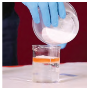
Green Rhino® CG1 Polymer is added. The spill is solidified.
